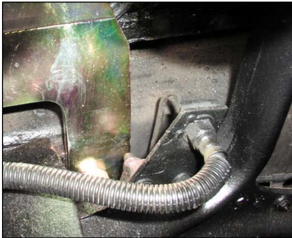
Photo 11 Check to be sure that the brake line is not touching the inner riser.
