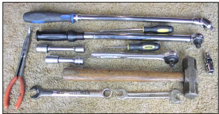
Photo 9 “Extra” tools found useful when removing and replacing the bolts that hold the bogie to the frame
