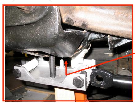
Insert 5/8 - 13 x 2 1/2" HH bolt and 5/8" lock washer into stop channel from the bottom and engage into locking block from inside the boggie. The Lock block has 5/8-13 nut welded on it and should be positioned with the nut up. Make sure the lock block is positioned to achieve maximum surface contact inside the boggie cavity.
