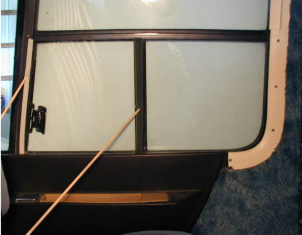
Picture 1: Remove the bottom screw in the window trim (next to the armrest). Note: this screw may need to be replaced with a longer one once the screen rail is in place. Then remove the tape from two foam pieces and place one on each vertical member of the window frame (shown by the pointers in the photo).
